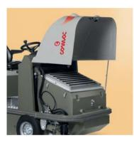
A fabric bag filter, with a large filtering surface - 7 sq.m (CS80) - 8 sq.m (CS90-CS110) - lasts a very long time and ensures excellent results even in environments where there is a lot of fine dust thanks to the powerful filter shaker. The filter is easy to remove without the use of tools, to check or replace it. No maintenance is required thanks to the periodical use of the electric filter shaker. Filters in fabrics for specific applications are available upon request
